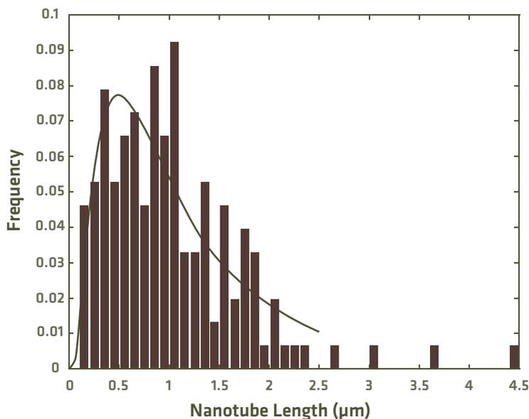
**Figure 6.** Atomic-force microscopy (AFM) data indicates that our SWNTs range in length from approximately 100 nm to 4 microns. A. B. C. Length histograms of our IsoNanotubes-M, IsoNanotubes-S, and PureTubes, respectively.
